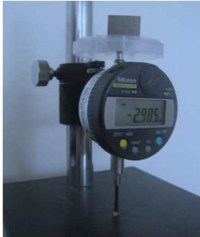
Figure 1. The Apparatus measures displacement for a known application of force.
